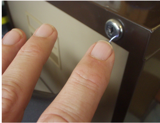
Figure 1. Captured on film! An electrostatic spark from a person's finger to a filing cabinet. The effects of electrical current passing through the human body are covered at length in the International Standard IEC 479-2:1987. It indicates that the energy content of a spark from the human body is too low to produce a direct serious risk to health. However case histories have shown a number of accidents due to shock reaction or recoil. Such accidents include falling down stairs and dropping or releasing loads.
