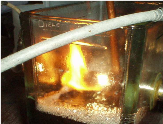
Figure 2. Electrostatic ignition of kerosene foam at 25C - fifty degrees below its flashpoint.
