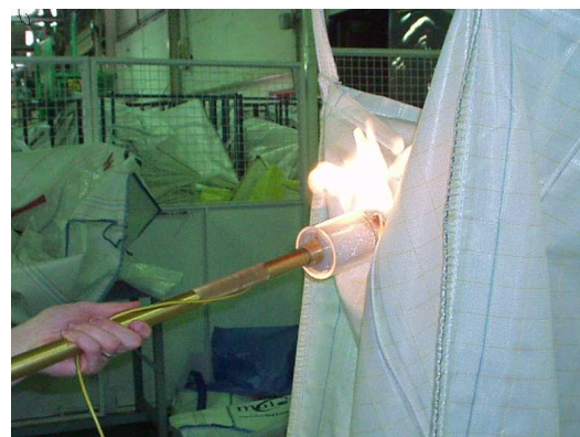
Figure 7. Propane ignition by brush discharge from an FIBC.
